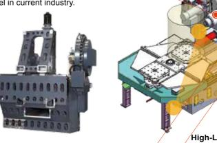
Symmetrical column design greatly reduce the effects of thermal displacement.
