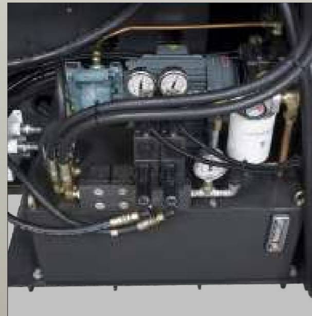
Worktable Hydraulic Brake Unit
